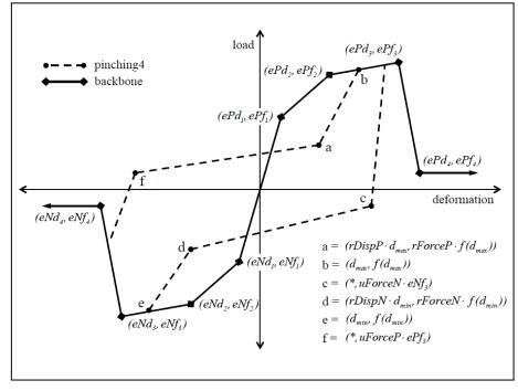
Figura 4.8 - Modelo multilinear *Pinching4*
